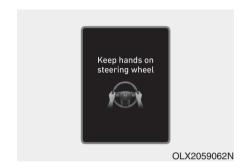
If the driver takes their hands off the steering wheel for several seconds while the LKA system is activated, the system will warn the driver.
