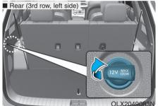
The power outlet is designed to provide power for mobile telephones or other devices designed to operate with vehicle electrical systems. The devices should draw less than 180 W with the engine running.
