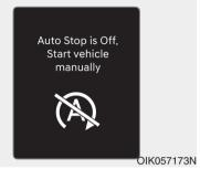
If the message "Auto Stop is Off. Start vehicle manually", appears on the LCD display with a beep sound, restart the vehicle manually by depressing the brake pedal with the vehicle shifted to P (Park) or N (Neutral). For your safety, restart the vehicle in the P (Park) position.
