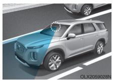
The Lane Keeping Assist (LKA) system helps detect lane markers on the road with a front view camera at the front windshield, and assists the driver's steering to help keep the vehicle between lanes.
