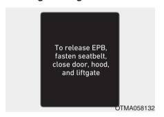
To release EPB, fasten seatbelt, close door, hood and liftgate
