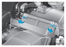
2. Pull down the lever (2) to the UNLOCK position.
