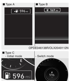
The range is the estimated distance the vehicle can be driven with the remaining fuel.
