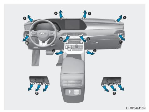
The mode selection button controls the direction of the air flow through the ventilation system. Air can be directed to the floor, dashboard outlets, or windshield. Five symbols are used to represent Face, Bi-Level, Floor, Floor-Defrost and Defrost air position.
