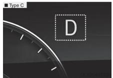
This indicator displays the gear position of the shift button.
