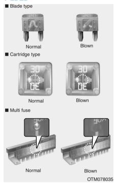
A vehicle's electrical system is protected from electrical overload damage by fuses.
