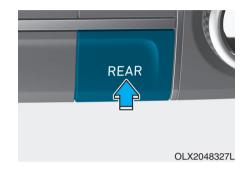
If you press the rear climate control button, rear passengers can control the rear climate system.
