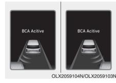
The Blind-Spot Collision-Avoidance Assist (BCA) system may apply braking power, when an approaching vehicle is detected within a certain distance next to or behind your vehicle.
