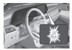
Front passenger's seat belt warning As a reminder to the front passenger, the front passenger's seat belt warning lights will illuminate for approximately 6 seconds each time you place the ignition switch to the ON position regardless of belt fastening.
