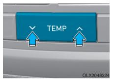
The temperature of delivered air can be set to the desired temperature by pushing the temperature control button.
