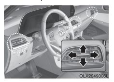
The instrument panel vent air flow can be directed up/down or left/right using the vent adjustment lever.
