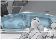
Curtain air bags are located along both sides of the roof rails above the front and rear doors. They are designed to help protect the heads of the front seat occupants and the rear outboard seat occupants in certain side impact collisions.
