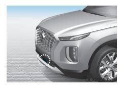
The Smart Cruise Control uses a sensor to detect distance to the vehicle ahead.
