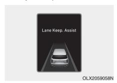
To see the LKA system screen on the LCD display in the cluster, select Assist mode (♠). For more details, refer to "LCD Display Modes" in chapter 3.
