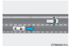
BCW system will alert you when it detects a vehicle is approaching in an adjacent lane at a high rate of speed. If the driver activates the turn signal when the system detects an oncoming vehicle, the system sounds an audible alert.
