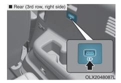
The battery charging state may be monitored on the electrical device. Disconnect the USB cable from the USB port after use.
