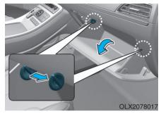
With the glove box open, remove the stoppers on both sides to allow the glove box to hang freely on the hinges.
