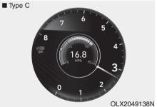
The tachometer indicates the approximate number of engine revolutions per minute (rpm).
