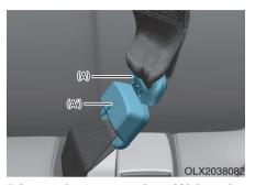
Insert the tongue plate (A) into the buckle (A') until an audible "click" is heard, indicating the latch is locked. Make sure the belt is not twisted.
