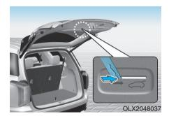
Your vehicle is equipped with an emergency liftgate safety release lever located on the bottom of the liftgate inside the vehicle.
