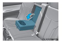
The armrest is located in the center of the rear seat. Use the strap in the center of the armrest to pull it down.
