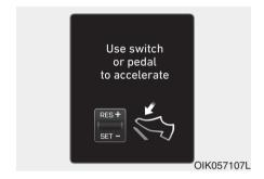
Use switch or pedal to accelerate While the Smart Cruise Control (SCC) system is operating, your vehicle stops behind the vehicle in front when it stops. The message shown above is displayed on the cluster within 3 seconds after the stop and the system will be in the standby position.
