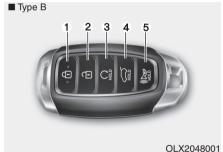
Your HYUNDAI uses a Smart Key, which you can use to lock or unlock the driver and passenger doors or the rear liftgate.
