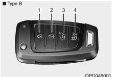
Your HYUNDAI uses a remote key, which you can use to lock or unlock the driver and passenger doors or the rear liftgate.
