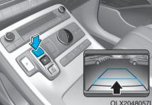
The Rear View Monitor will activate when the engine is running and the shift button is in the R (Reverse) position.
