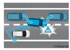
The Blind-Spot Collision-Avoidance Assist (BCA) system helps detect the front lane through the camera installed on the upper front wind-shield and helps detect the side/rear areas through radar sensors.
