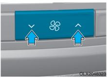
The fan speed can be set to the desired speed by pushing the fan speed control button. The higher the fan speed is, the more air is delivered. Pressing the OFF button turns off the fan.
