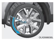
7. Loosen the wheel lug nuts counterclockwise one turn each in the order shown above, but do not remove any lug nuts until the tire has been raised off of the ground.
