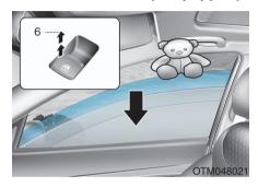
If a window senses any obstacle while it is closing automatically, it will stop and lower approximately 12 inches (30 cm) to allow the object to be cleared.
