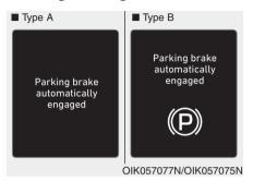
Parking brake automatically engaged
