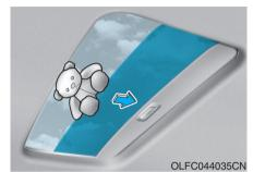
If the sunroof senses any to an obstacle while it is closing automatically, it will reverse direction then stop to allow the object to be cleared.
