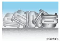
Front air bags may not inflate in rollover accidents because air bag deployment could not provide protection to the occupants.
