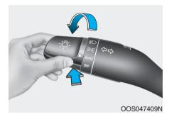
The High Beam Assist (HBA) is a system that automatically adjusts the headlamp range (switches between high beam and low beam) according to the brightness of other vehicles and road conditions.
