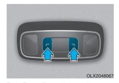
Rear Room Lamp ( >> <<: >: Press either buttons to turn the room lamp on or off.
