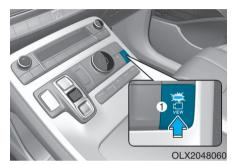
The Surround View Monitoring system can assist in parking by allowing the driver to see around the vehicle. Push the button (1, indicator ON) to operate the system. To cancel the system, push the button again (1, indicator OFF).
