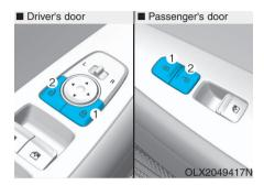
The driver side and front passenger side door armrest is equipped with a central door lock switch. The lock button is indicated by a  $(\stackrel{\frown}{\square})$  symbol. The unlock button is indicated by a  $(\stackrel{\frown}{\square})$  symbol.
