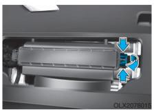
3. Remove the climate control air filter case while pressing the lock on right side of the cover.
