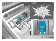
With the driver's door and engine hood closed, depress the brake pedal and then press the [AUTO HOLD] switch. The white AUTO HOLD indicator will come on and the system will be in the standby position.
