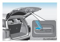
Your vehicle is equipped with an emergency liftgate safety release lever located on the bottom of the liftgate inside the vehicle.
