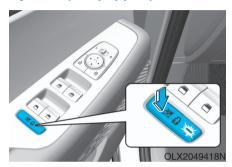
If you push the Electronic child safety lock switch and the indicator illuminates, rear passengers cannot open the rear door from inside the vehicle. To cancel the Electronic child safety lock system, push the Electronic child safety lock system switch one more time and then the indicator turns off.
