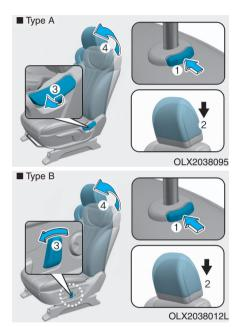
To reinstall the head restraint:
