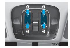
Front Room Lamp (1) ( \( \): Press the button to turn the front and rear room lamps on or off.
