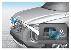
3. Go to the front of the vehicle, raise the hood slightly, push up the secondary latch (1) inside of the hood center and lift the hood (2). After it has been raised about halfway, it will raise completely by itself.
