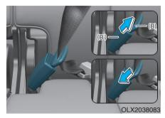
Pull out the tongue plate (B) from the pocket. Pull the tongue plate (B) and insert it into the buckle (B') until an audible "click" is heard, indicating the latch is locked. Make sure the belt is not twisted.
