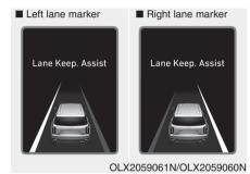
A visual warning appears on the cluster LCD display. Either the left lane marker or the right lane marker in the cluster LCD display will blink depending on which direction the vehicle is veering. Also, the steering wheel will vibrate.
