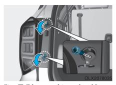
Stop/Tail lamp and turn signal lamp (Type A)
