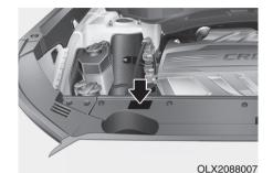
Air Conditioning refrigerant label You can find out which air conditioning refrigerant is applied to your vehicle on the label located in front of engine compartment.
