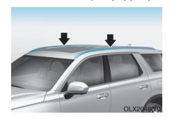
If your vehicle comes equipped with roof side rails, then roof rack cross-bars can be installed on top of your vehicle.
