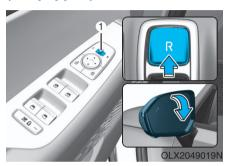
When you move the shift button to the R (Reverse) position, the side view mirror(s) will rotate downwards to aid with driving in reverse. The position of the side view mirror switch (1) determines whether or not the mirrors will move:
