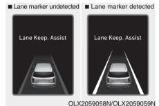
If vehicle speed is over 40 mph (64 km/h) and the system detects lane markers, the color changes from gray to white.
