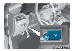
To apply the EPB (Electronic Parking Brake):
