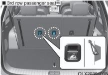
First secure the child restraint with the LATCH lower anchors or the seat belt. If the child restraint manufacturer recommends that the top tether strap be attached, attach and tighten the top tether strap to the top tether strap anchor. Child restraint hook holders are located on the rear of the seatbacks.
