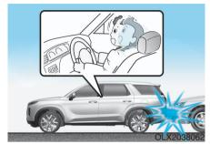
Front air bags are not designed to inflate in rear collisions, because occupants are moved backward by the force of the impact. In this case, inflated air bags would not provide any additional benefit.
