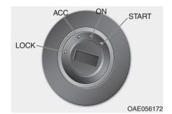
Whenever the front door is opened, the ignition switch will illuminate, provided the ignition switch is not in the ON position. The light will go off immediately when the ignition switch is turned on or go off after about 30 seconds when the door is closed. (if equipped)
