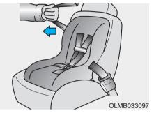
Pull the shoulder portion of the seat belt all the way out. When the shoulder portion of the seat belt is fully extended, it will shift the retractor to the "Automatic Locking" (child restraint) mode.
