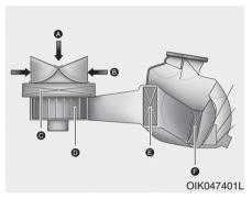
[A] : Outside air, [B] : Recirculated air [C] : Climate control air filter, [D] : Blower
