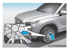
6. Insert the tool (1, if equipped) into the hole and pull out the wheel cover.
