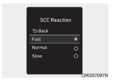
The sensitivity of vehicle speed when following the front vehicle to maintain the set distance can be adjusted. Go to the 'User Settings → Driver Assistance → SCC Reaction → Fast/Normal/Slow' on the LCD display. You may select one of the three stages you prefer.
